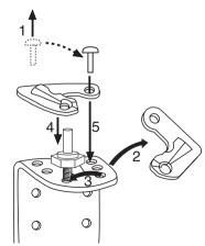
4. Remove the door fitting on the lower right (1) and reposition the door hinge bracket cover from the lower left to the right of the door (2), place the door fitting supplied in the lower left of the door (3). Carefully remove the door to the front and place on one side.
